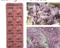
PTP sheet (left) separated into plastic (top right) and aluminum foil (bottom right)
