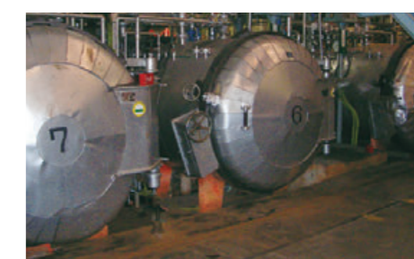
Original retort pressure cookers—pressure and heat sterilization at high temperature enables long shelf life without the use of preservatives
